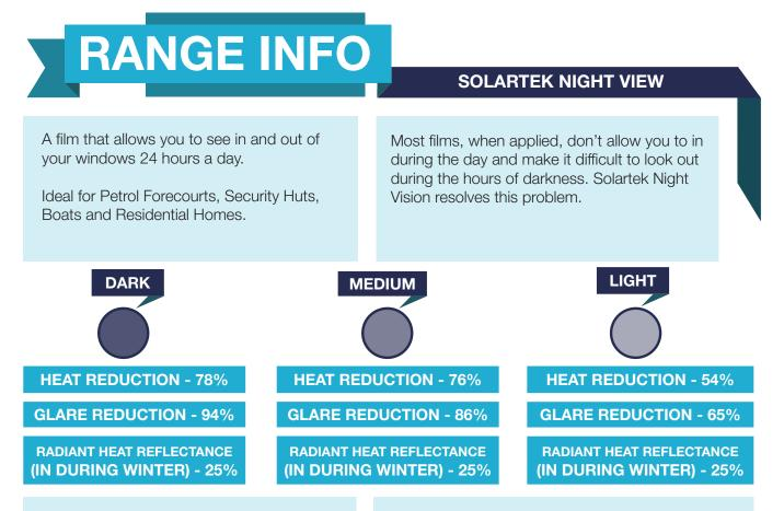
Night Vision window films help block the sun's damaging UV rays, reduce glare and reject the sun's heat.
