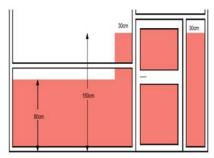
\*Glazing in Bathing Areas – any glazing forming part of a bath or shower screen, or located adjacent to, or surrounding a bath, swimming pool, or other associated wet area constitutes a potential danger because of the possibility of a slip accident.
